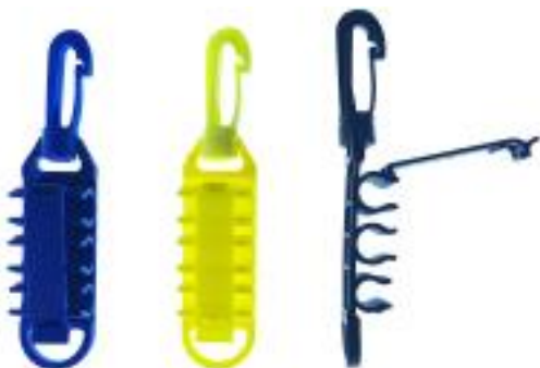
Hose clamp - AH-09 Fits three hoses. Two big grooves for 9/16" (14 mm) hose. One small groove for 1/2" (12.5 mm) hose.
