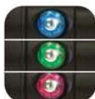
Battery level indicator built-in: Blue color / Green color / Red color / Flash Red color
